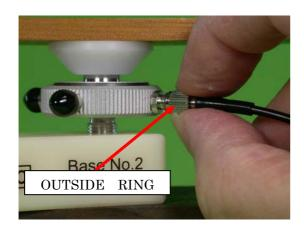
Screw the outside ring of the **output cable** to fix it to the **output connector** of the **sensor**.
