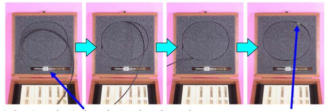
At first, insert the <u>1/4 phone plug</u> into the cushion and snap the cables into the grooves of the cushion in sequence as shown in the picture.
