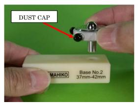
Then put the sensor into the selected base, screwing it into the hole of the base until the bottom part of the sensor touches on the surface of the base.
