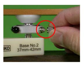
Then turn **the sensor** part left to pull it up until the **contact chip** *lightly* touches the soundboard and stop it. Remember which **output connector** (any one out of four) faces in approximately best direction for cable connection.
